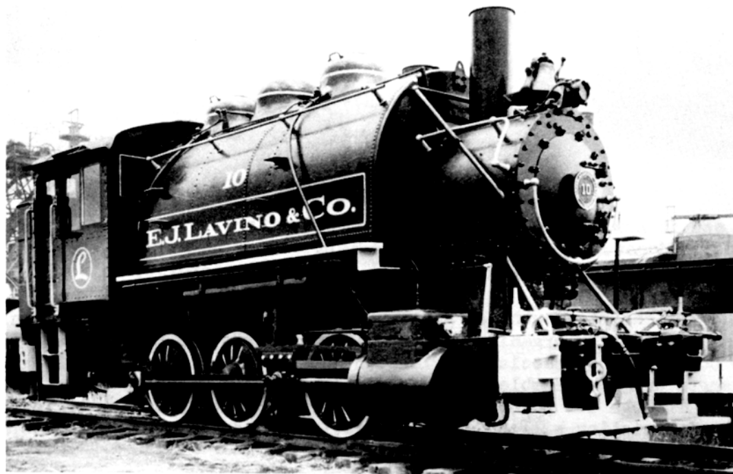
Steam Locomotive No. 10 - donated to the Museum by Owner E. J. Lavino and Company, Sheridan, Penna. It is an 0-6-0 (tank) coal burner built in 1923 by Alco. (R. D. Crompton picture)
