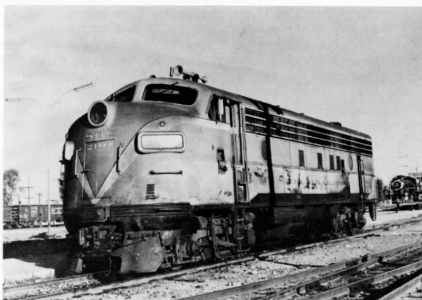
Steam boilered FP7 No. 2101 is the yard switcher in Benjamin Hill, and is shown here backing down to the depot. Steam loco in the background is a 1909 Baldwin product on display between FCP and S-BC rails that bracket the station.
